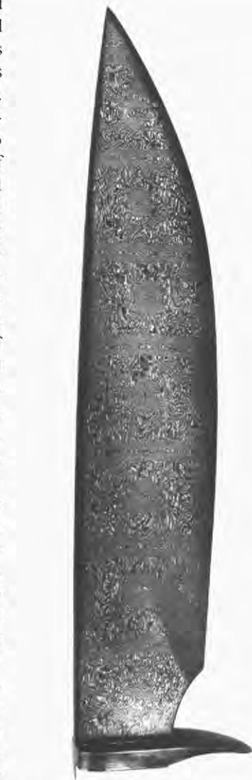
Figure 4. A reconstructed Damascus blade containing a combined Mohammed ladder + rose pattern. Ferric chloride etch (full size)
