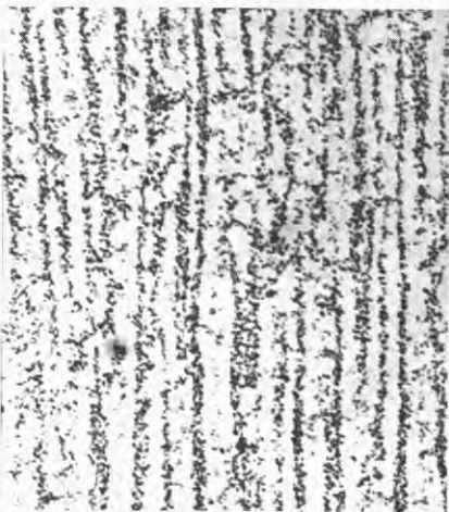
Figure 3a. Transverse section of figure 2 blade. Etched in boiling picric to produce dark cementite in white pearlite matrix ( \times 100 )
