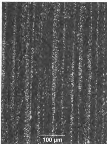
Figure 5. Longitudinal section of figure 4 blade showing bands of cementite particles that the surface pattern. Nital etch
